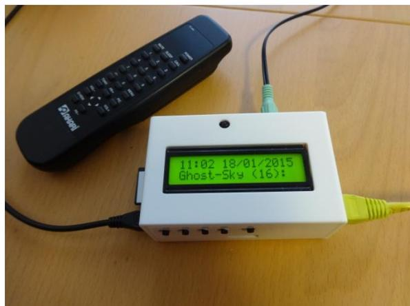
Figure 21 PiFace CAD Radio with IR Remote Control
