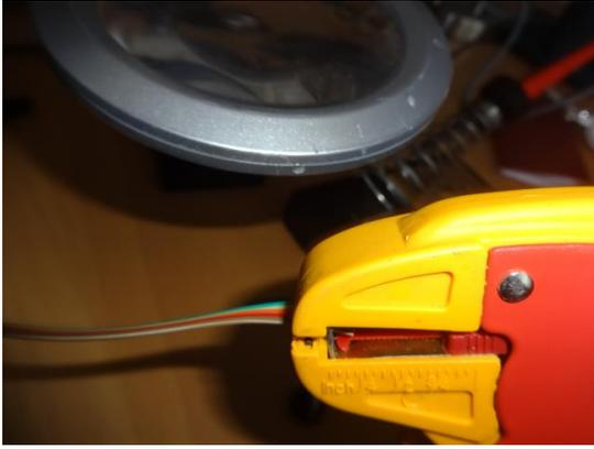
Figure 112 Using wire strippers
