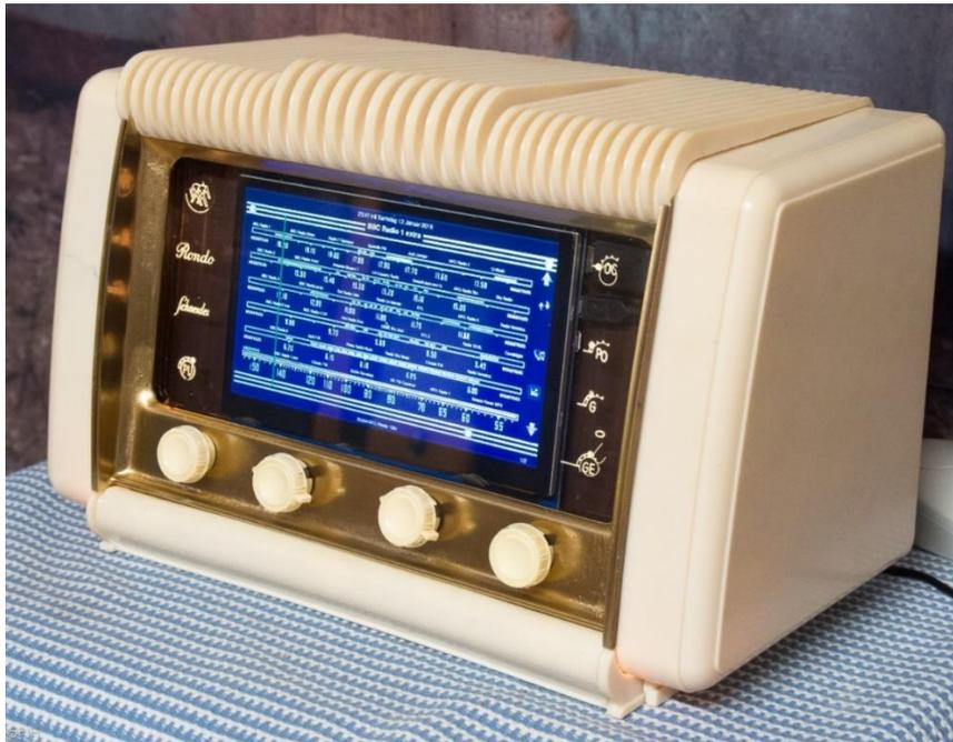
Figure 25 Vintage radio using a touch screen
