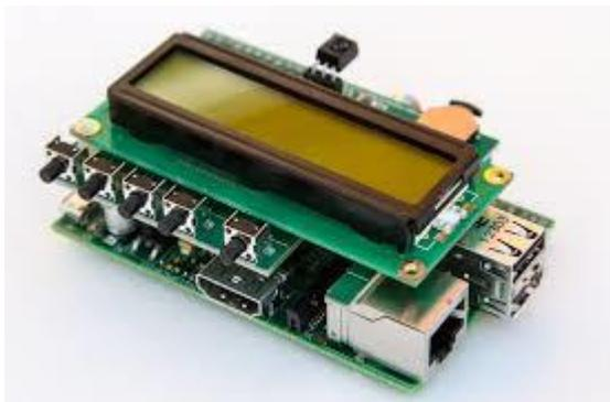
Figure 109 PiFace CAD and Raspberry PI
