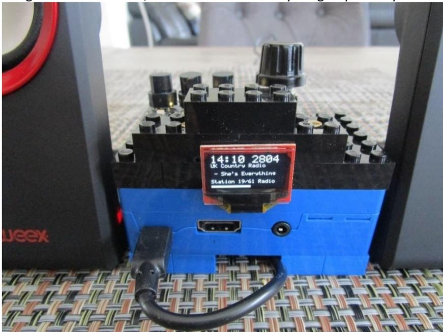
Figure 108 Lego radio with IQaudIO Cosmic controller and OLED
