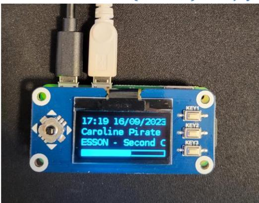
Figure 46 RPi 1.3" 128x64 OLED with joystick
