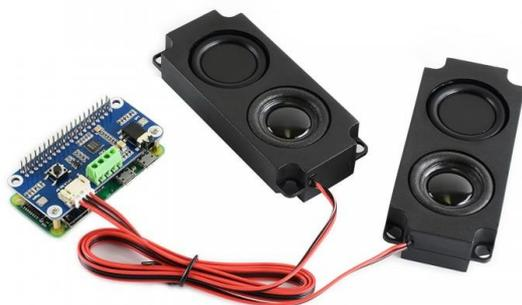
These cards are often sold with a pair of speakers which plug directly into the card. The particular speakers shown are 5W enclosed speakers.
