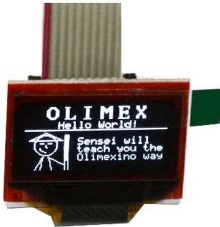
The Olimex 128x64 pixel OLED is a low cost, low power, high contrast LCD display with a UEXT connector. It is controlled via the I2C or SPI interface. The power supply required is only in the range of 1 uA in sleep mode, 200 uA in operating mode and 7mA in display ON mode. View area is 21 x 11 mm. It is particularly useful where space is very limited.
