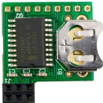
Figure 241 RasClock RTC V4.2 module
