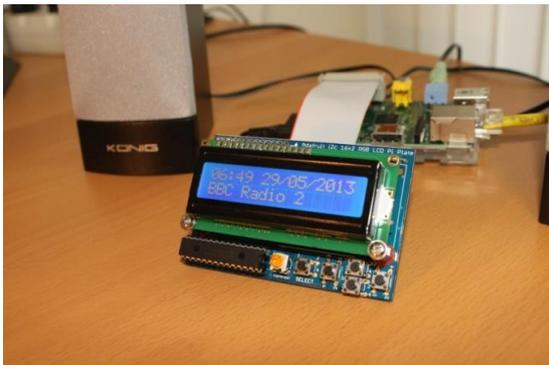
Figure 6 Radio using the Adafruit LCD plate
