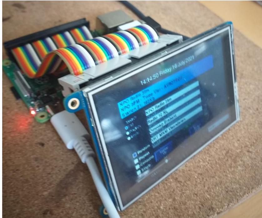
Figure 66 TFT connected by a 40-pin male/female ribbon cable
