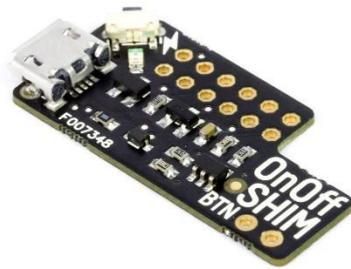
Figure 239 Pimoroni On-Off shim power switch
