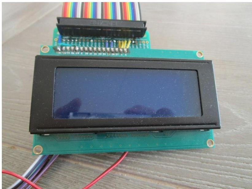
Figure 89 Interface board with LCD screen attached
