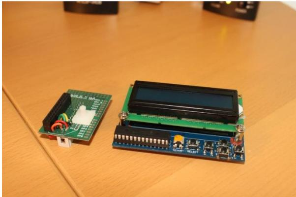
Figure 93 Adafruit LCD plate
