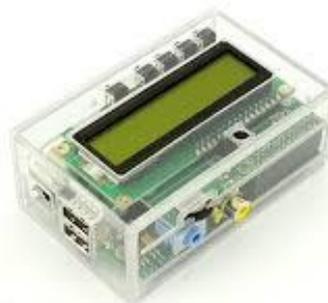
Figure 110 PiFace CAD in a case
