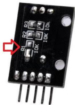
Figure 77 KY040 Missing 10K resistor
