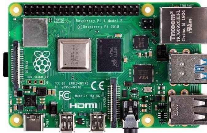
Figure 29 Raspberry Pi Model 4B Computer
