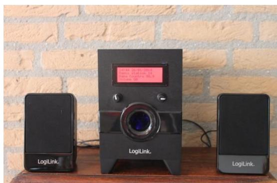
Figure 8 Pi radio using rotary encoders
