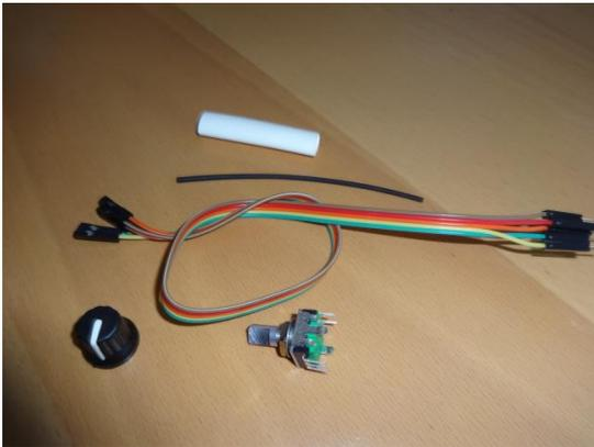
Figure 111 Rotary encoder wiring components
