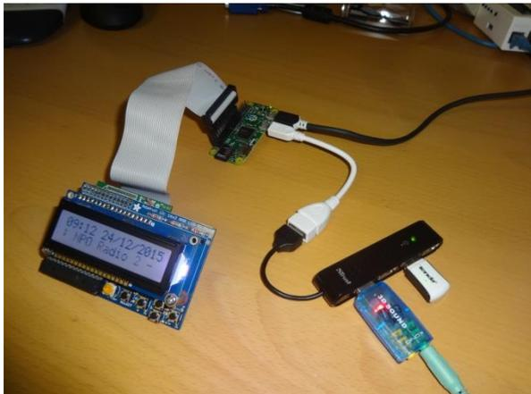
Figure 12 The Radio running on a Pi Zero
