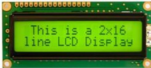
Figure 37 The HD44780U LCD display
