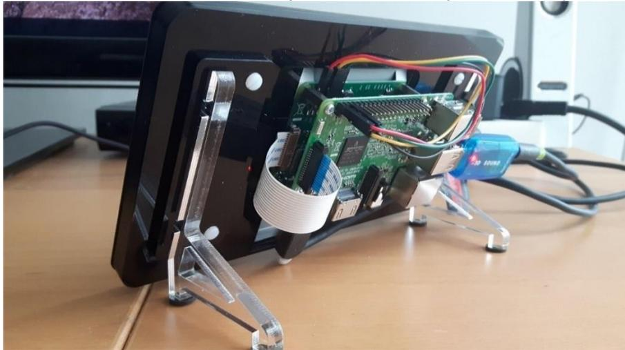
Figure 63 Raspberry Pi 3 with 7-inch touch screen
