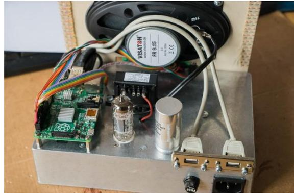
Figure 19 The RPi valve radio chassis view
