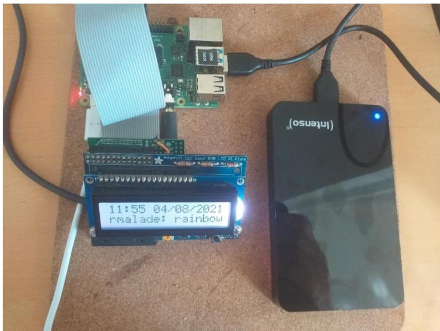
Figure 236 Raspberry Pi booting from an Intenso USB 3.0 2.5-inch disk drive
