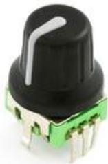
This project originally uses a COM-09117 12-step rotary encoder or PEC11R series encoders. It also has a select switch (by pushing in on the knob). These are “Incremental Rotary Encoders”. An incremental rotary encoder provides cyclical outputs (only) when the encoder is rotated. The other type is an absolute rotary encoder which maintains position information even when switched off (See Wikipedia article on rotary encoders).
