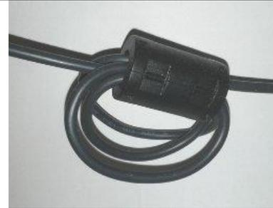
Figure 124 Loop +5V supply around the core
