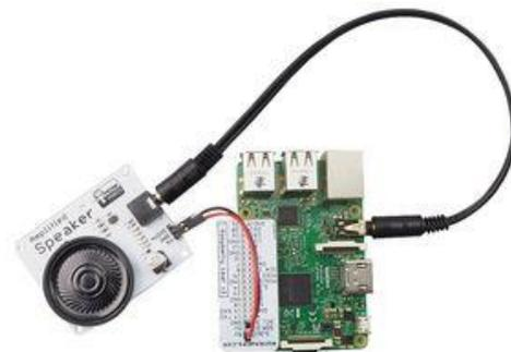
Figure 122 Audio output jack amplifier
