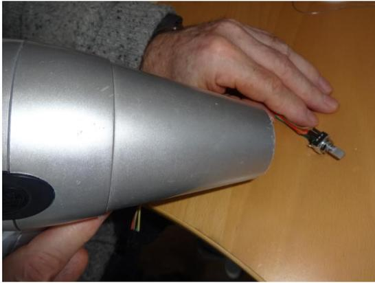
Figure 115 Shrink shrink-wrap with a hair dryer
