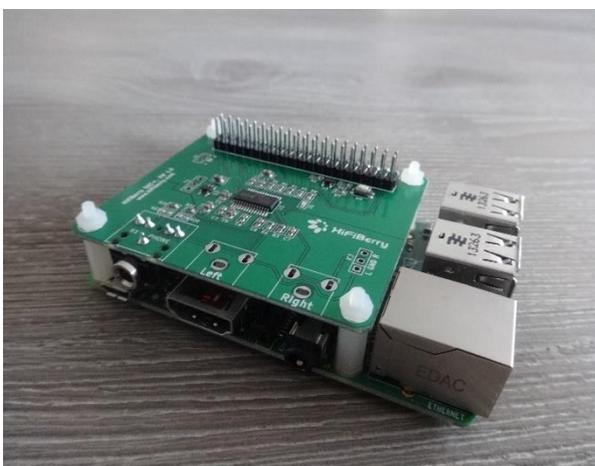
Figure 48 HiFiBerry mounted on the Raspberry Pi
