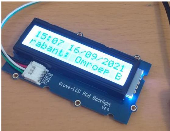
Figure 45 Grove LCD RGB Backlight
