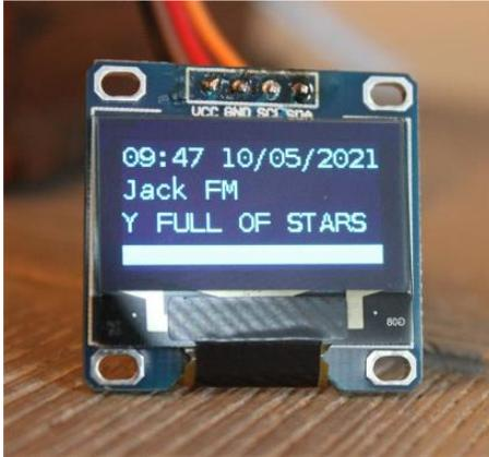
Figure 42 Sitronix SSD1306 128x64 pixel monochrome OLED
